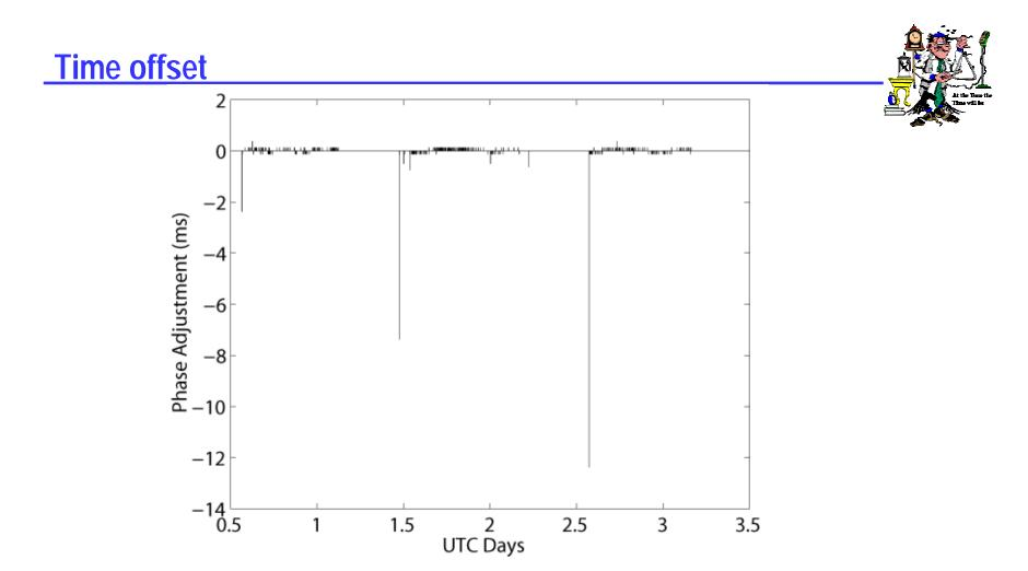
• Note the spikes when the time offset is computed as the signal comes up. This can happen if the oscillator has drifted since last set or because the comb filter has not stabilized.
