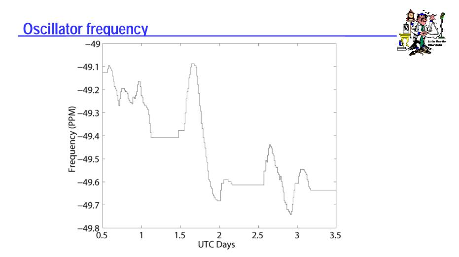
• Note the periods when the oscillator frequency is a horizontal line. This happens when the signal is lost and the oscillator is coasting at its last determined frequency.
