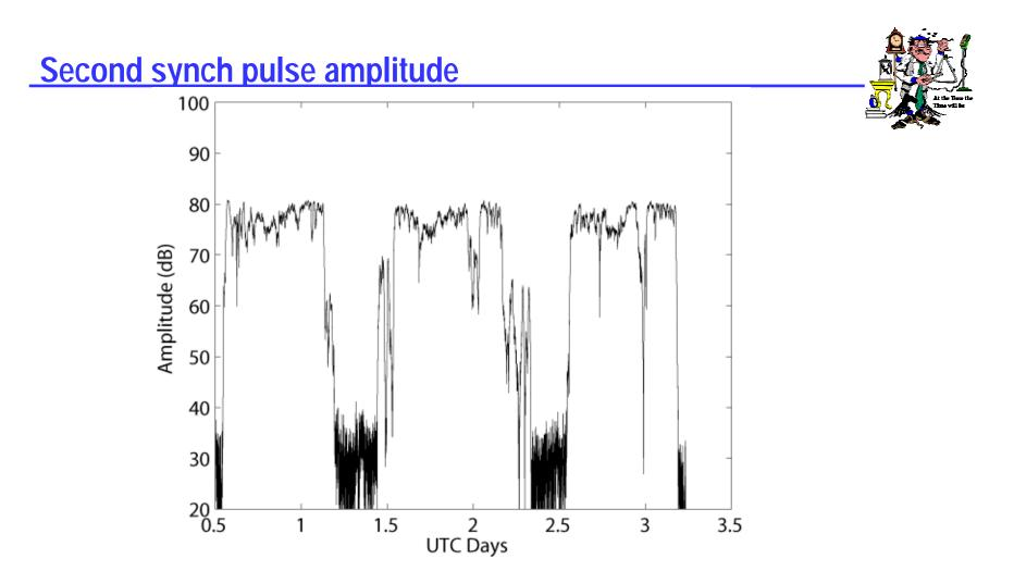
• This is the master time reference for the driver. It is also the most sensitive to oscillator wander and severe signal multipath.
